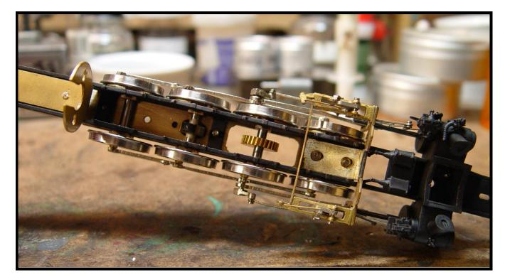
This view "inside" the frame shows the clean burnished upside surface of the new bottom plate. The GME sound cam is clearly shown on the third axle; -- selected as a choice location given the room to fit the contact slider inside the frame and out of harm's way if installed beneath the bottom plate. Above the left cylinder is the lubricator left missing by NPP, and in the center of the cylinder saddle are the brake cylinders similarly omitted by NPP.
