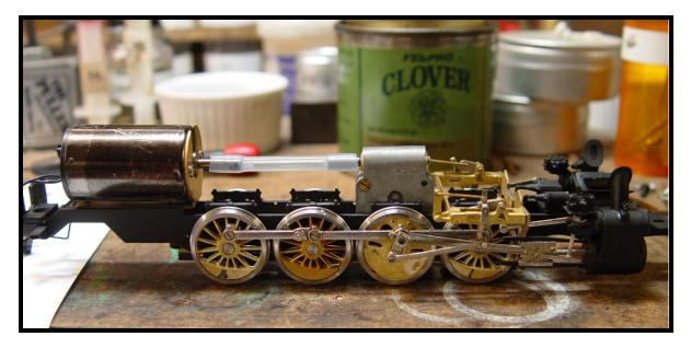
Here the motor and new gearbox are installed. In this application a short piece of model airplane fuel line is used as shown; -- though not yet completely aligned. Notice that, in order to keep the very limber fuel line from "whipping" about, I insert a piece of rod into the tubing. The ends remain flexible enough to absorb some shock and serve in place(s) of universals....but then without the need to craft an additional torque arm device for the gearbox body.
