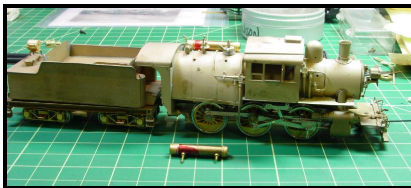
Here is an O&W Class V 2-6-0 rebuilt from a NPP Class U 2-6-0; -- 63” drivers, cut down steam chest and raised cab profile.....newly fabricated footboard pilot—all in an early stage of construction.
