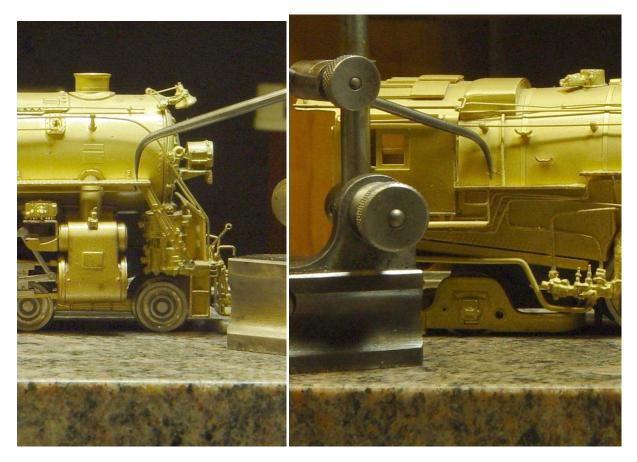
After some measurements with calipers it appears that running boards are correctly placed, but comparisons with a surface gauge suggest that the boiler – superstructure is the trouble. That can be resultant from either too low a mounting point at the rear of the cab, or that the cylinders are seated in the frame at too high up in the frame saddle.
