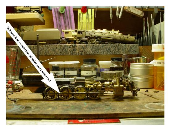
In this much rebuilt Y-2 mechanism the side rod, at center, lines up with the piston rod, as it should be! The alteration here involved lowering the entire cylinder set, through a tedious trial and error, to arrive at the proper and correct alignment. Noticeable also is the additional detail of the brake cylinders, centered on the frame immediately to the rear of the cylinder saddle.
