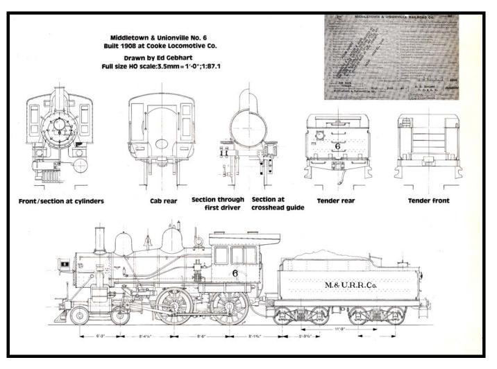
While altered from an "original" appearance, especially with the addition of Inside Admission Baker Valve Gear and the "top story" of an enlarged valve chamber to accommodate revised slide valves for operation under Superheat, this is nearly the configuration of the other Class A engines as they appeared in O&W service.
