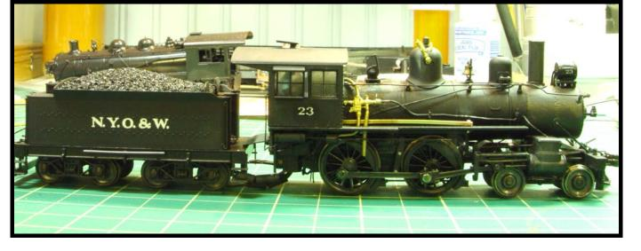
Here in a nearly completed form is the "converted" Richmond engine, made over into the Cooke Works O&W locomotive. For this image I've left the details yet unfinished and unpainted so that they may be more clearly seen by the reader.
