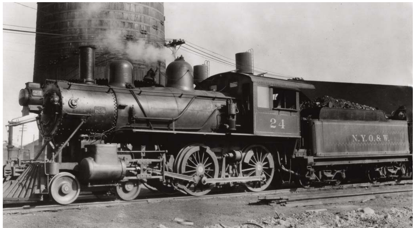
This image shows No. 24 in an early configuration at Middletown (with the Dodge Coal Trimmers just visible in the left background), with it yet to receive and electrified headlamp, as witnessed by the lack of a turbo generator between the steam dome and cab front.
